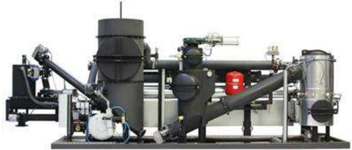
Down-draft gasifier coupled with IC engine
